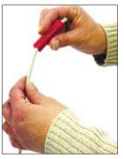
2 Slide Shrink Tube 3 Use Heat Gun To Sleeve Over Wire, 3 Shrink Material Cable. Tube Or **Round Object**
