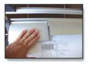
1. Punch the holes in your document sheets with the Stripbind Machine. The split punching system allows for easy punching. Punches 20 pages.
