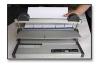
3. Position the document in the closing mechanism of the Stripbinder Machine. Document is held in a special grooved edge to allow easy binding.
